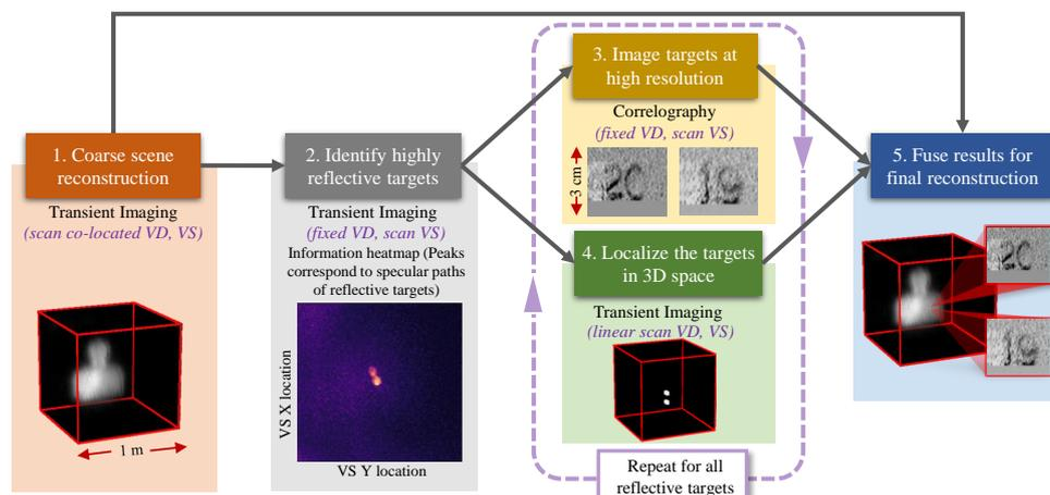
Fig. 2. Pipeline for foveated non-line-of-sight imaging
